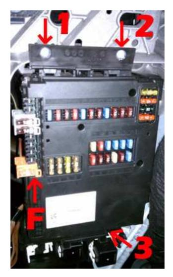
4) Then with the screws removed from the rear of the SAM, the front edge will unclip from the relay board at the "3" location pictured above.
